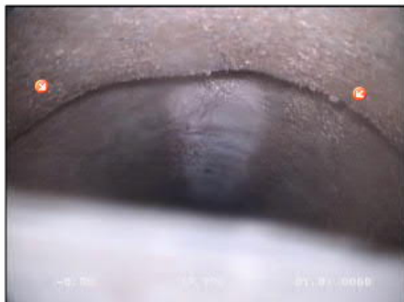
Photo: 7_7_20_A.JPG 21,2m, Fissure circulaire
