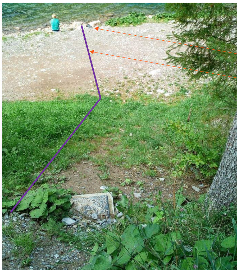
Figure 6 – Implantation canal de fuite DN400
