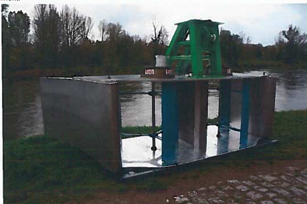
Figure 1-10. Hydrolienne HYDROQUEST RIVER 1.40 avant installation
